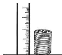
Fig. 1.2: Determination of the thickness of a coin
