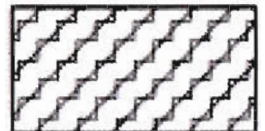
(I) Thermal insulation
