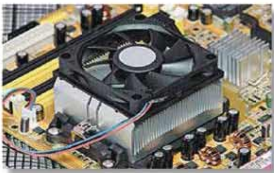
Fan is set over the processor to keep it cool
