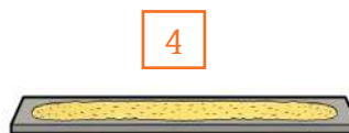
The cold solution is poured to separate the crystals. It is then dried by pressing in a dry sheet or filter paper.
